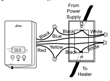
Attach wires per diagram above.
